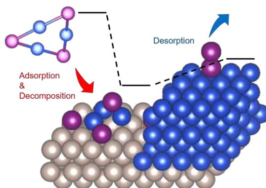
Fig. 1: Molecular mechanism of LPCVD of Cu.
