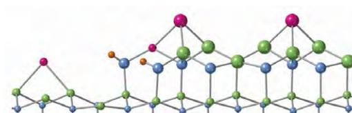
Fig. 3: The GN step-edge structure with two NH units intervening in the Ga-Ga bonds. Burgandy, green, blue and orange balls depict Ga adatom, Ga, N and H atoms, respectively.
