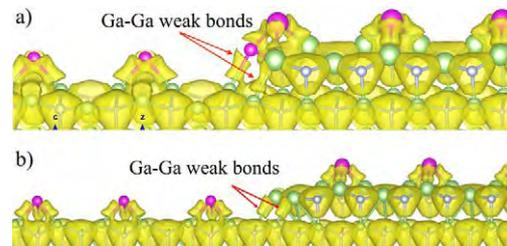
Fig.1: Calculated electron densities near the GN step (a) and the Ga<sub>2</sub> step (b). The densities are represented by the yellow isovalue surfaces. The small yellow clouds reflect the presence of the low electron density, indicating that the Ga-Ga weak bonds are formed at the step edges. The Ga, Ga-ad (Ga adatom), and N atoms are represented by the green, pink, and blue balls, respectively.
