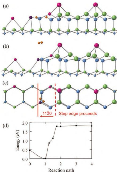
Fig.4: An elementary process in the step-flow growth of GaN. (a) Stable structure of the GN step edge attached with 2 NH units and an additional Ga atom nearby. (b) Stable structure of the GN step with H<sub>2</sub> desorbed from the structure (a). (c) The top view of the stable structure shown in (b). Color code of the balls depicting atoms are the same as in Fig. 3. The additional Ga adatom is shown by purple. (d) Calculated energy profile for the reaction from (a) to (b).
