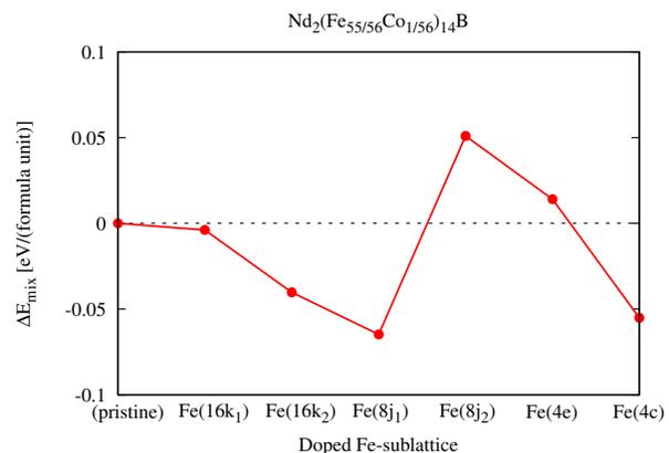
Figure 1: Calculated mixing energy of Co and Nd<sub>2</sub>Fe<sub>14</sub>B.
