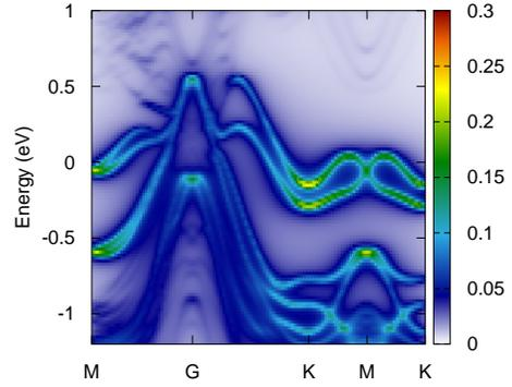
Figure 3: Calculated surface state of Bi-terminated YPtBi. The intensity spectra are calculated by projecting the band onto the 10 atomic-layer unit cell.
