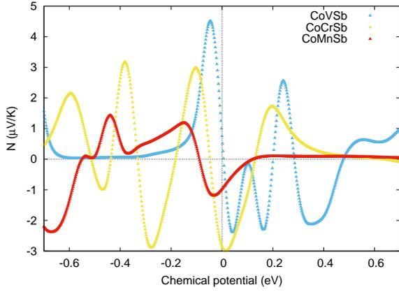
Figure 2: Anomalous Nernst coefficient at 300K. The Fermi energy is set to 0 eV.
