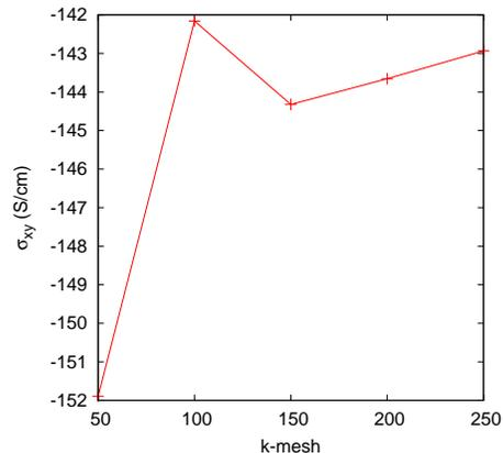
Figure 1:  $k$ -mesh dependence of anomalous Hall conductivity  $\sigma_{xy}|_{T=0}$  for CoVSb at Fermi energy.  $\sigma_{xy}$  are calculated by using  $k \times k \times k$  mesh in the Brillouin zone.
